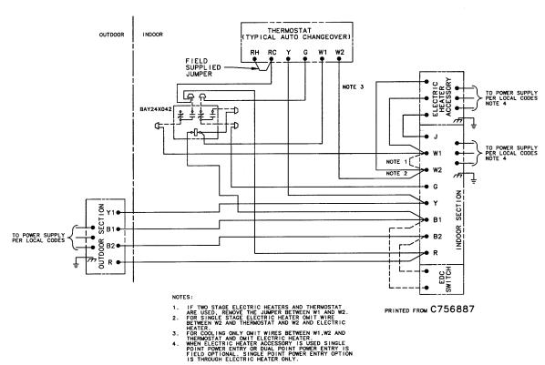
Figure 15. TTA090A, 120A/TWE090A, 120A; TTA075A, 100A/TWE075A, 100A
